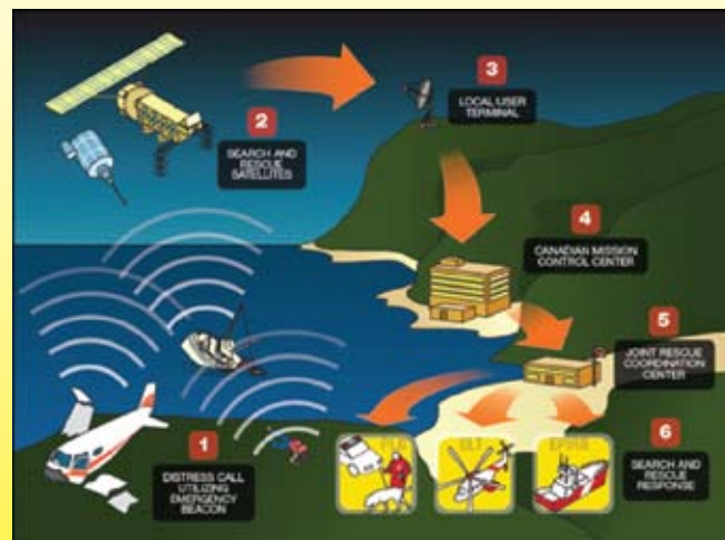
Fig. 1 – How the COSPAS-SARSAT system works.
